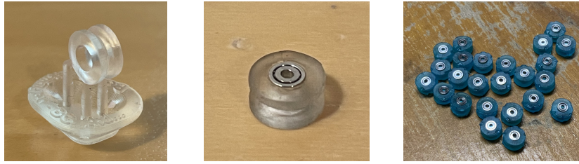
Figure 4: Finger tendon pulley made from clear SLA printing material. Left image shows the pulley with support structure after the printing, middle image shows the pulley assembled. The right image shows the pulley made from blue, tough SLA printing material (right).
